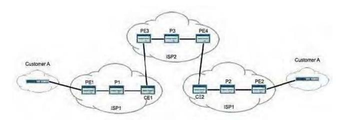
Customer A wants a Layer 3 VPN between their two sites. To support this, you purchase a carrier-ofcarriers solution from ISP2. Referring to the topology in the exhibit, how many labels does PE1 push onto data packets destined for PE2?
