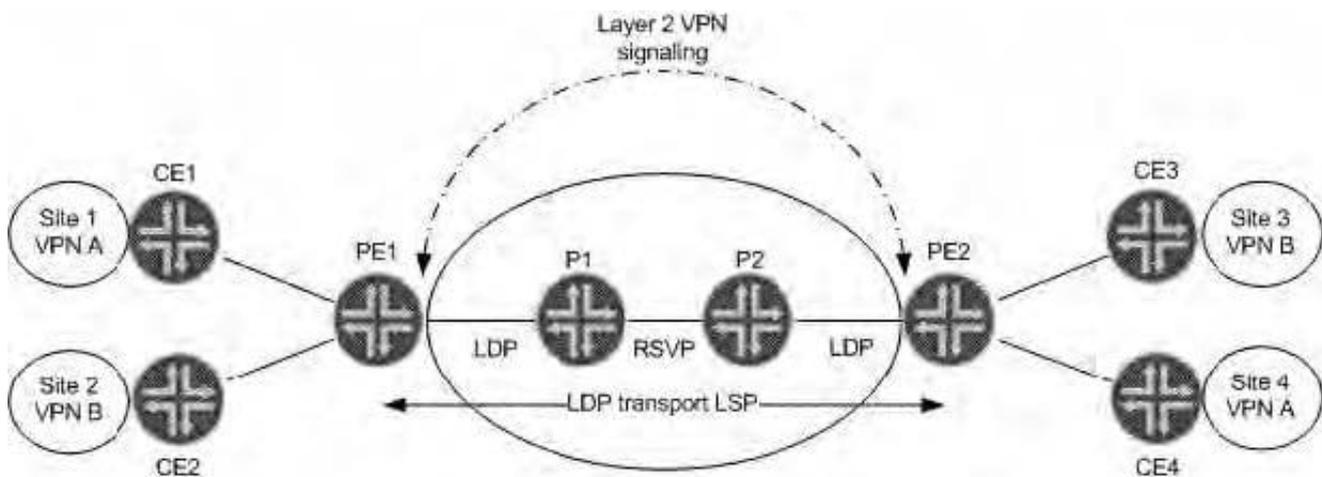
A LDP Layer 2 circuit is shown for VPN A and VPN B. LDP tunneling over RSVP is activated on P1 and P2. Referring to the exhibit, which statement is true about the LDP Layer 2 circuit?
