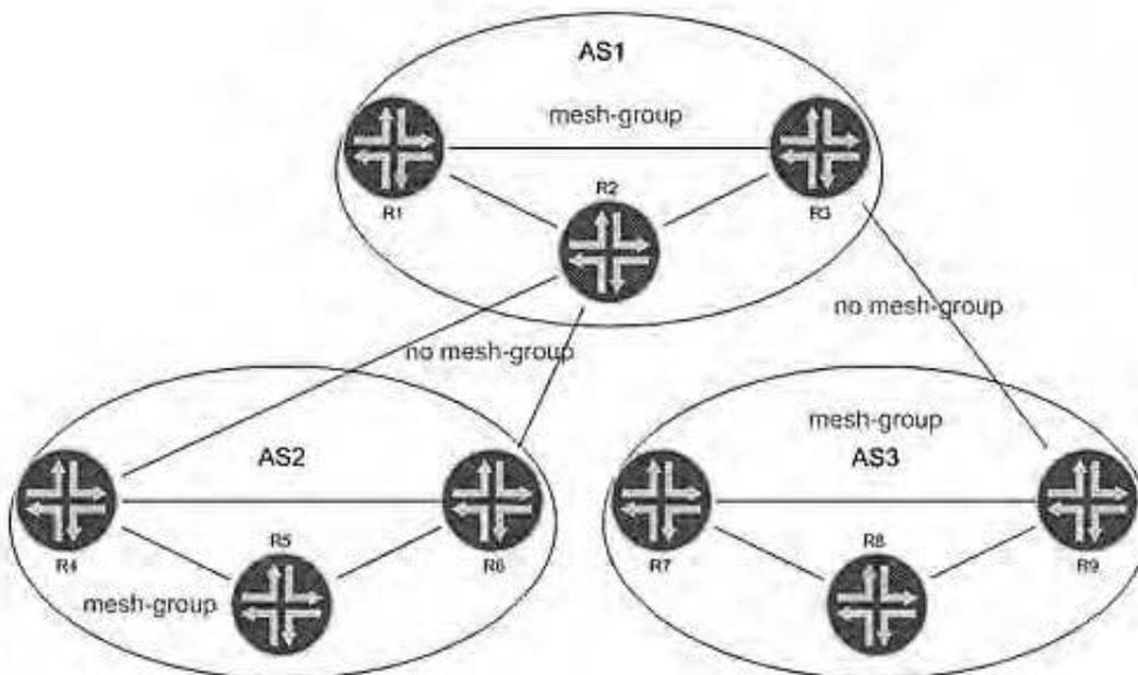
In the exhibit, all routers within each AS are configured for Anycast RP. All intra-AS routers are configured within the same MSDP mesh group. Inter-AS multicast has been enabled using MSDP without MSDP mesh groups. Which statement is true?
