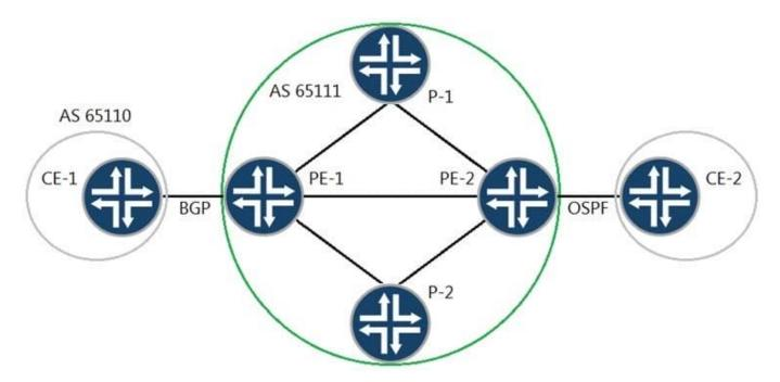
You have a Layer 3 VPN established between PE-1 and PE-2 to allow communication between CE-1 and CE-2. You want to establish communication between CE-1 and CE-2.
