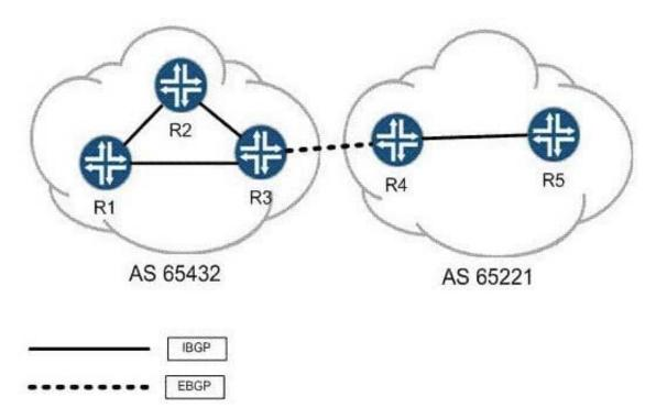
R3 and R4 want to establish an EBGP session between each other\\'s loopback addresses. Static routes have been configured for the loopback addresses and you can ping from loopback to loopback. Their EBGP sessions are configured with multihop to allow for additional hops. The correct AS numbers have been specified at the [routing-options] hierarchy as well. Considering the topology in the exhibit, which statement is true?
