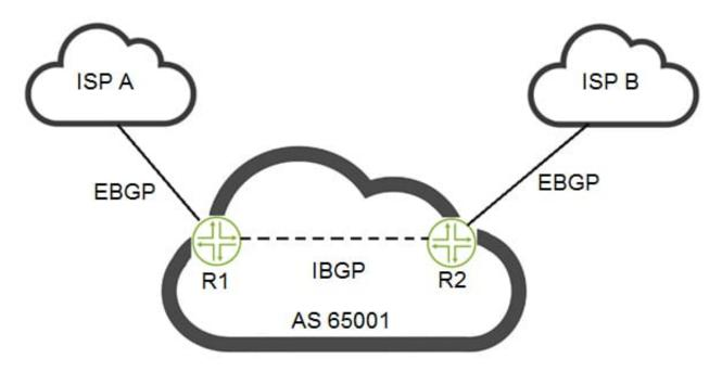
You are configuring BGP policies for a site with a dual-homed connection as shown in the exhibit. You must ensure that inbound traffic from Internet hosts flow through the ISP A connection.
