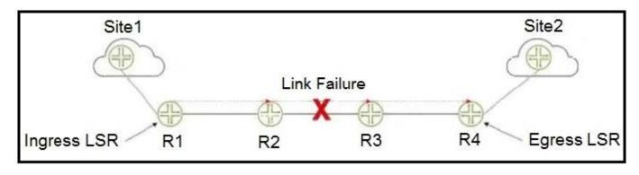
Referring to the exhibit, you have an established RSVP LSP between R1 and R4 when you experience a link failure between R2 and R3. Which two statements are correct? (Choose two.)
