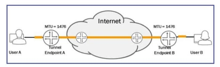
You have created a GRE tunnel as shown in the exhibit. The router with tunnel endpoint A is dropping the packets originating from User A and destined to User B.
