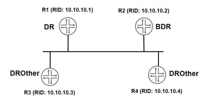
You have configured OSPF routing as shown in the exhibit. You notice that all interfaces have formed full adjacencies, with the exception of the interfaces connecting R3 and R4 with a status of 2Way.
