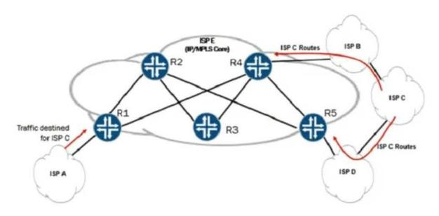
A. Apply the BGP import policy (to EBGP peers) on R4 anaVor R5 to adjust the local preference on the ISP C routes so that the path through ISP B is more preferred
