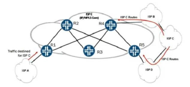
A. Apply the BGP import policy (to EBGP peers) on R4 anaVor R5 to adjust the local preference on the ISP C routes so that the path through ISP B is more preferred
