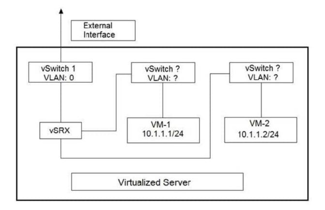
You are designing the virtualized server deployment shown in the exhibit in your data center. The vSRX device is acting as a Layer 2 firewall and the two VMs must communicate through the vSRX device.
