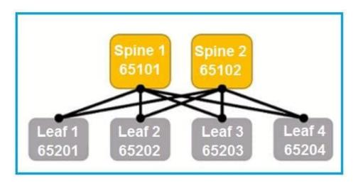
For a fully configured and functional IP fabric underlay as shown in the exhibit, how many external BGP neighbors are expected to be in established state for Leaf 1?
