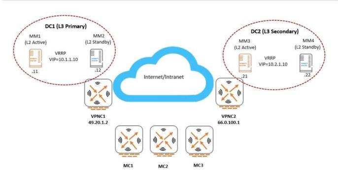
(MC2) #show running-config | include masterip Building Configuration... masterip 10.1.1.10 vpn-ip 19.20.1.2 ipsec aruba123 peer-id xx:xx:xx:xx:xx:xx secondary masterip 10.2.1.10 vpn-ip 66.0.100.1 ipsec-factory-cert vpn-mac-1 xx:xx:xx:xx:yy:yy interface vlan 140 (MC2) #■
