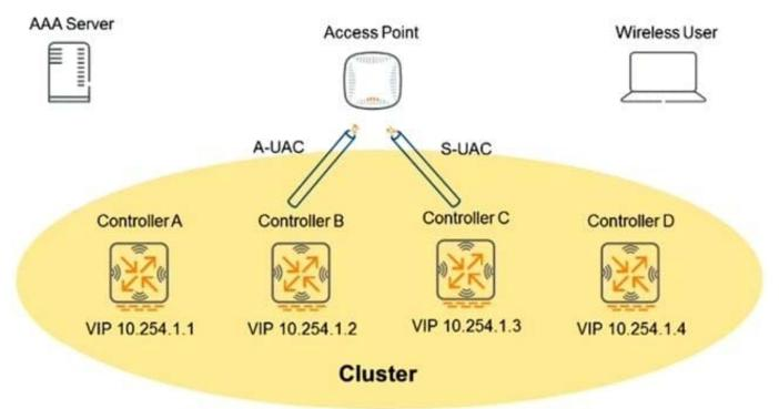
An AP is connected to a cluster of controllers. An AAA server provides all authentication and authorization functions for wireless users. A wireless user connects to an AP, and Active User Anchor Controller (AUAC) and Standby UAC (S-UAC) tunnels are built from the AP to the respective controllers in the cluster.
