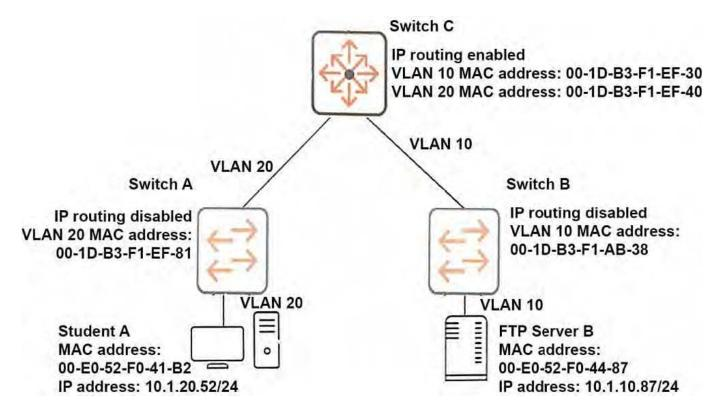
The student A client needs to connect to FTP Server B. Student A sends the necessary ARP request and receives a reply.
