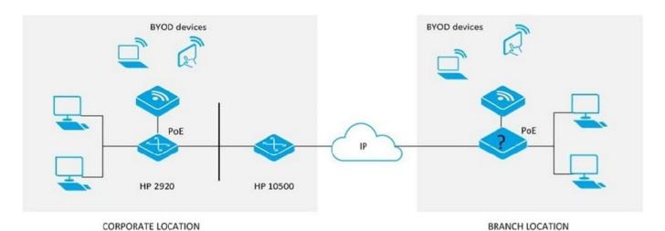
A company wants to connect a mid-size branch office to their corporate location. An HP 10500/7500 Unified Wired-Wireless module is deployed at the corporate location. A maximum of six HP MSM access points will be deployed at the branch location.
