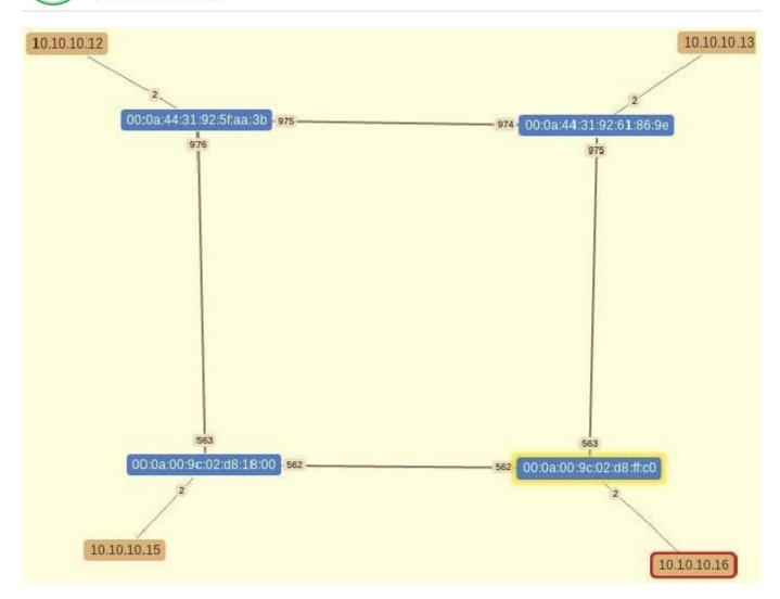
The switches in the diagram are connected to each other using two physical cables. The network consists of two HP 3800 series switches and two HP 5900 series switches. Why is only one link displayed between switches in the OpenFlow Topology diagram on the HP VAN SDN Controller?
