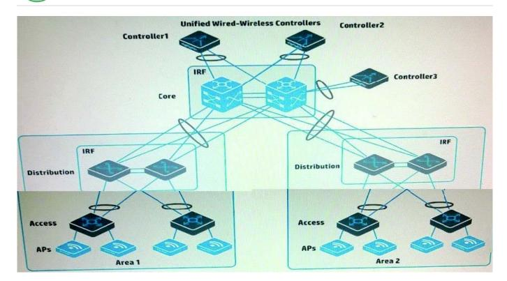
A company has two HP Unified Wired-Wireless controllers. The MSM APs in Area 1 in the exhibit are controlled by Controller1. The MSM APs in Area 2 in the exhibit are controlled by Controlled. The company purchases a Controlled to provide backup for both Controller1 and Controller2 (N+1 redundancy).
