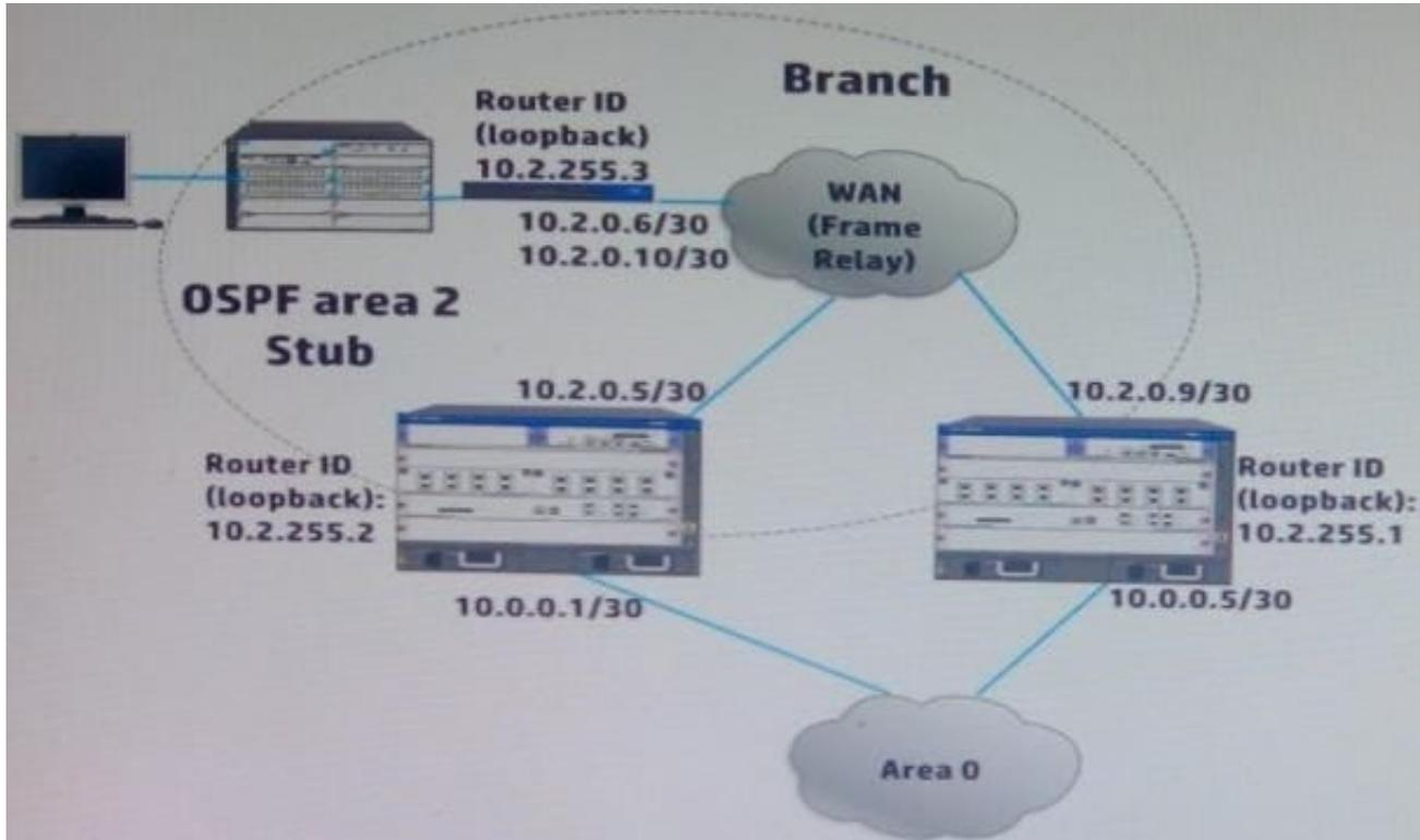
The branch routers have E1 lines into the Frame Relay Service provider network. The exhibit shows just one branch, but the network actually has 30 branches. The HP 6600 Series routers, which are the area border routers (ABRs), have E2
