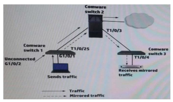
A network administrator up a remote mirroring on the HP Comware switches in the exhibit. The administrator must define several port while entering mirroring- group commands on these switches. Which port should be the reflector port
