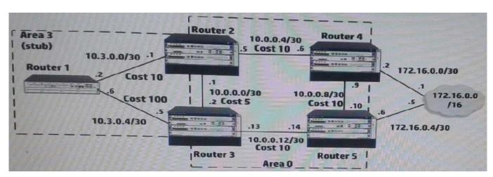
Router 4, which is an HP Comware router, redistributes Routing Information Protocol (RIP) routes into Open Shortest
