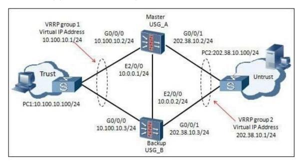
When USG\_A is in failed state, such as power failure, this time USG\_B state switched from Slave to Master.
