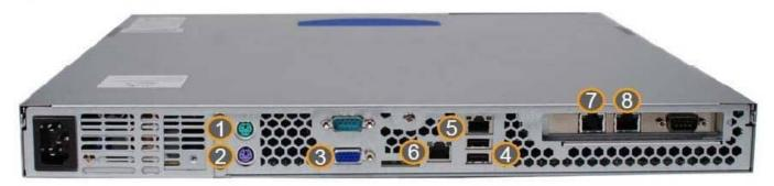
Which cable should be connected to the VMAX Service processor illustrated as \\'5\\'?
