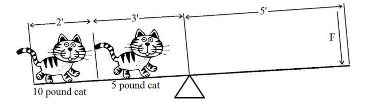
The amount of force (F) needed to balance the lever in the figure above is most nearly \_\_\_\_\_\_
