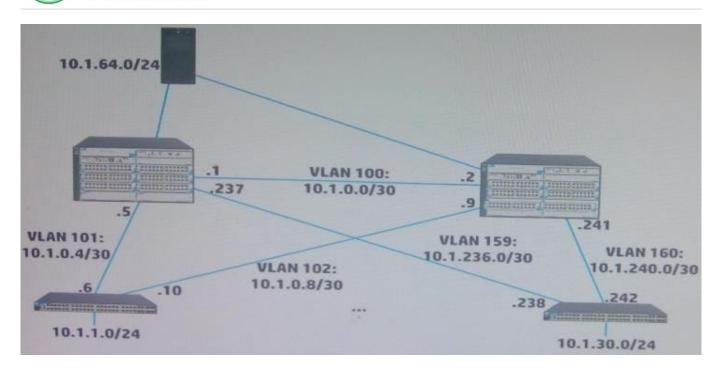
The exhibit shows the topology for a network with 30 access layer switches (only two are shown). Every switch-to-switch link is a Gigabit link. Every virtual local area network (VLAN) interface runs Open Shortest Path First (OSPF) and has
