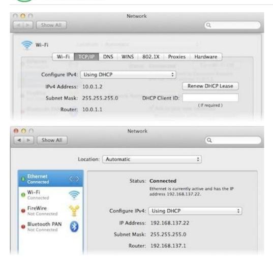
If a Mac with the network configuration shown above needs to initiate a connection to a server at address 17.20.8.9, which interface will it use to do so?
