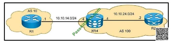
XR4 must protect itself from a DOS attack against its BGP process from R1 by using the TTL security feature. Which configuration achieves this goal?
