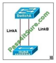
BPDUGuard is enabled on both ports of SwitchA. Initially, LinkA is connected and forwarding traffic. A new LinkB is then attached between SwitchA and HubA. Which two statements about the possible result of attaching the second link are true? (Choose two.)
