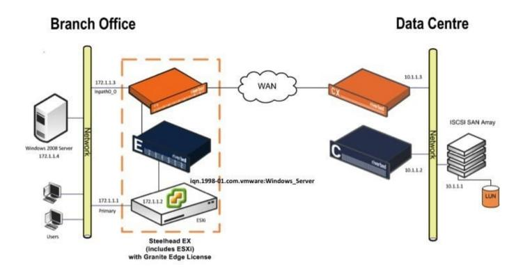
Step A. Granite Edge is configured to add the Granite Core. Step B. Granite Core discovers Granite Edge and ISCSI SAN. Step C. ISCSI San Administrator maps LUN to Granite Core. Step D. Granite Core discovers LUN and projects it
