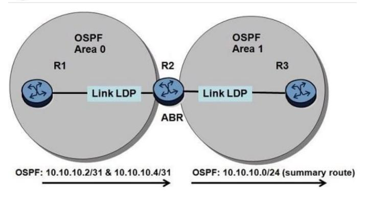
Router R2 advertises the aggregate prefix 10.10.10.0/24 into Area 1. Why would LDP aggregate-prefixmatch be enabled on router R3?
