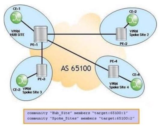
For the PE hub and spoke VPRN, on which PE(s) should the VPRN service command "vrf-target export target:65100:1 import target:65100:2" be configured?
