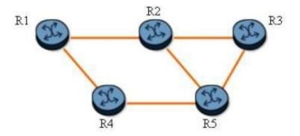
Two LSPs traverse the path R1-R2-R3. Both LSPs are configured with facility fast reroute and link protection. When router R1 is the PLR, which router becomes the Merge Point (MP) for this LSP?
