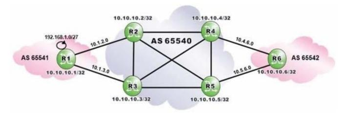
AS 65540 routers are iBGP fully-meshed. Assume routers R4, R5 and R6 are configured with addpaths ipv4 send 2 receive". Which routes to 192.168.0.1/27 is router R6 expected to have in its BGP routing table?
