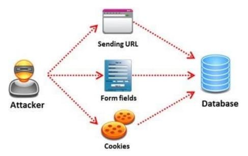
Pen tester needs to perform various tests to detect SQL injection vulnerability. He has to make a list of all input fields whose values could be used in crafting a SQL query, including the hidden fields of POST requests and then test them separately, trying to interfere with the query and to generate an error.
