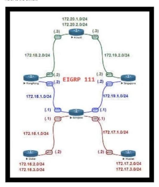
For Company XYZ Bangkok is using ECMP to reach the 172 20 2 0/24 network The company wants a design that would allow them to forward traffic from 172 16 2 0/24 toward 172 20 2 0/24 via the Singapore router as the preferred route The rest of the traffic should continue to use ECMP.
