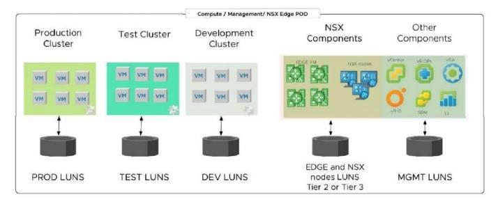
An NSX-T architect has been asked to review and recommend improvements for an NSX-T Data Center Logical Design, as shown in the drawing. The design must allow workload bursts for tenants to and from the public cloud and accommodate 30% yearly growth.
