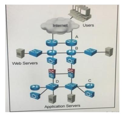
The operations team has identified that some of the multi-tiered e-commerce application have slow performance, due to illegitimate inbound traffic form the internet. On which device do you place traffic filtering to improve performance?
