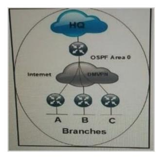
Each branch network must connect to the HQ and other branch networks over the phase 2 DMVPN network using a single tunnel interface. OSPF is running over the DMVPN network. Which network type is compatible with the DMVPN tunnel and ensures that the next hop of any route is unchanged?
