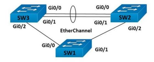
SW2# show etherchannel summary Flags: D - down P - bundled in portchannel I - stand-alone s - suspended H - Hot-standby (LACP only) R - Layer3 S - Layer2 U - in use f - failed to allocate aggregator M - not in use, minimum links not met u - unsuitable for bundling w - waiting to be aggregated d - default port Number of channel-groups in use: 1 Number of aggregators: 1 Group Port-channel Protocol Ports ----+---+----+----+----+----+---\_\_\_\_\_ 1 Pol(S D ) LACP G10/0(I) G10/1 (I)
