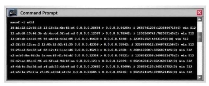
In MAC flooding attack, a switch is fed with many Ethernet frames, each containing different source MAC addresses, by the attacker. Switches have a limited memory for mapping various MAC addresses to physical ports. What happens when the CAM table becomes full?
