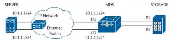
A high-availability setup for iSCSI is designed with the host running iSCSI multipath software. Each IP storage port on the MDS switch exports the same two Fibre Channel target ports with different iSCSI target names. In this design, how many iSCSI sessions are created from the host so that recovery occurs if any component fails?
