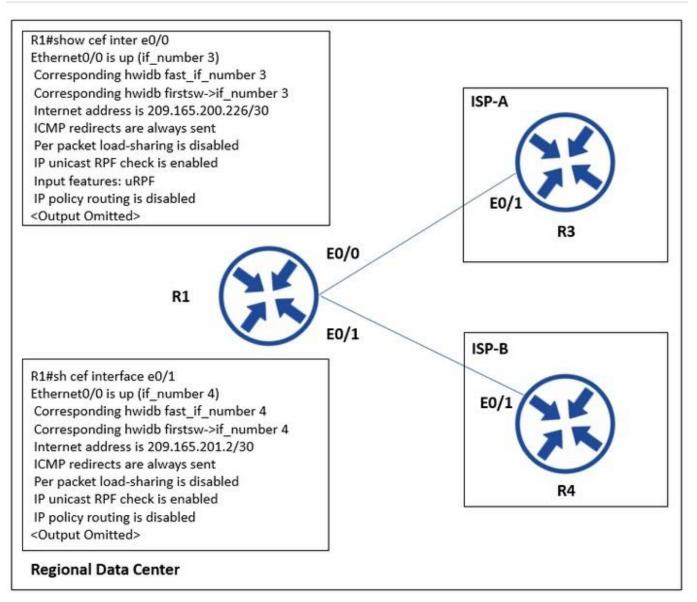
The company implemented uRPF to address an anti spoofing attack. A network engineer received a call from the IT security department that the regional data center is under an IP attack Which configuration must be implemented on R1 to resolve this issue?
