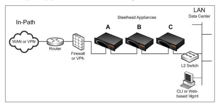
For connections initiated from the data center, there is a possibility that the Steelhead appliances shown in the exhibit will end up peering with each other, rather than the intended remote Steelhead appliances.
