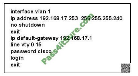
A network administrator has configured a Catalyst 2950 switch for remote management by pasting into the console the configuration commands that are shown in the exhibit. However, a Telnet session cannot be successfully established from a remote host. What should be done to fix this problem?
